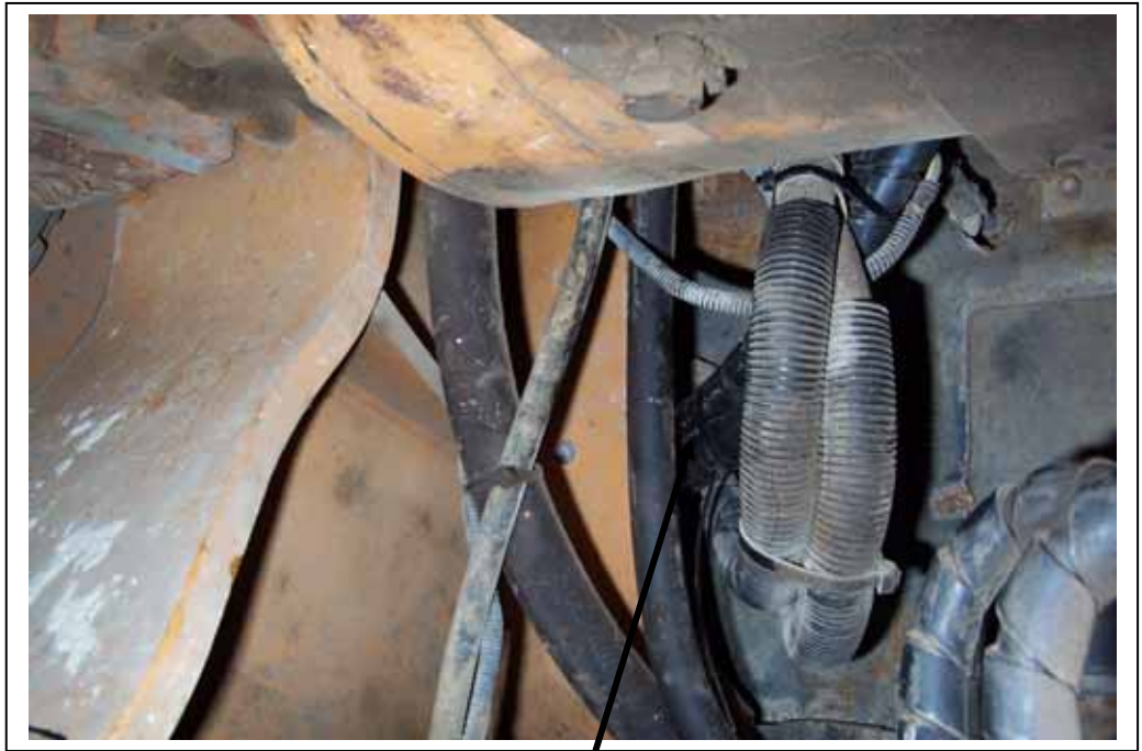
A/c Hoses and clutch wire entering cab beside heater lines
