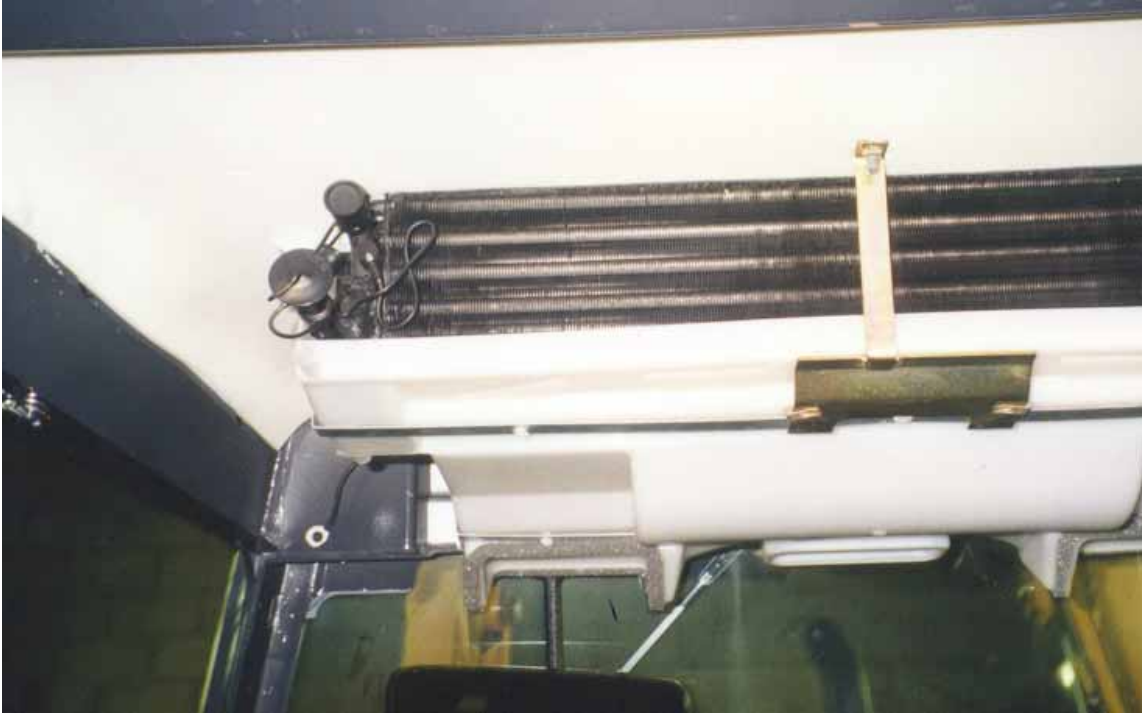
Fitting end of evaporator (left end).
