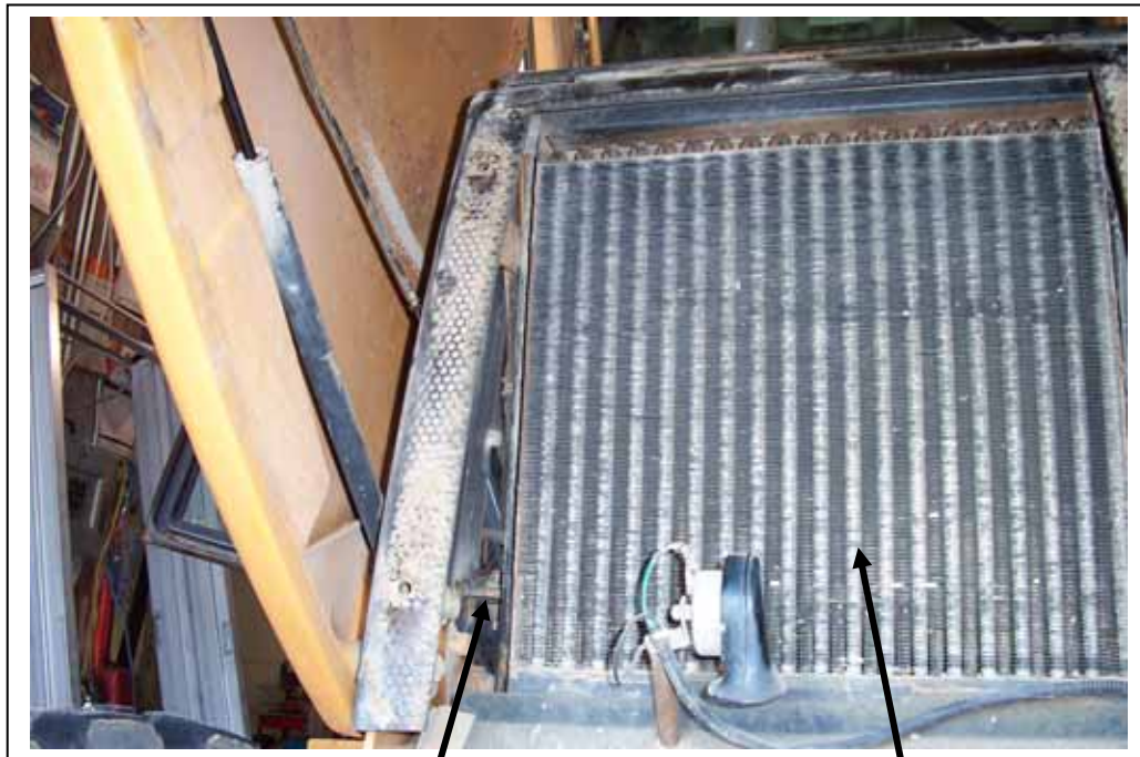
Foam removed from beside the rad frame
