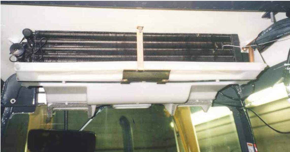
Evaporator mounted in position.
